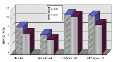
Figure 2 - Hot Modulus of Rupture Values for High Alumina Castables with Spinel Additives
