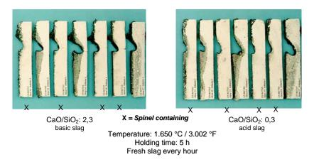
Figure 5 - Slag corrosion tests - induction furnace
