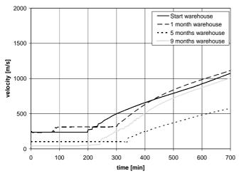
Fig. 2c. Ultrasonic graphs of NCC-AB / warehouse storage
