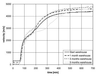
Fig. 2b. Ultrasonic graphs of LCC-ADS/W / warehouse storage
