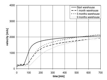
Fig. 2a. Ultrasonic graphs of LCC-PACA / warehouse storage
