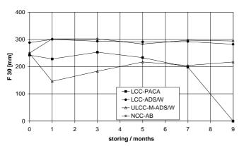
Fig. 3. Impact of warehouse aging on flow at 30 minutes
