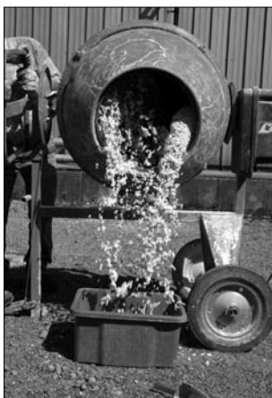
Fig. 2: VIB 8 E-SY in gravity mixer; no lump formation during mixing
