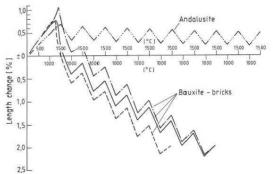
Fig. 4: Creep of andalusite and bauxite bricks tested under torpedo car application conditions; load 0.2 MPa, temperature change between 1000 and 1500  $^{\circ}$ C [27]
