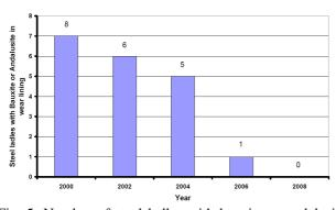
Fig. 5: Number of steel ladles with bauxite or andalusite based wear linings presented in international seminar on steel ladle lining in Europe 2000 – 2008 [32]
