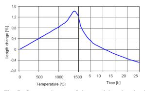
Fig. 7: Creep resistance of dense calcium hexaluminate, Bonite, based castable after pre-firing at  $1500 \text{ }^{\circ}\text{C} / 5 \text{ h}$
