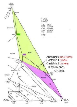
Fig. 11: Matrix composition of Andalusite based low cement castables with and without addition of fine matrix aluminas in the phase diagram  $CaO-Al_2O_3$ -SiO<sub>2</sub> [40]. Castable 2 with matrix aluminas, castable 1 without. HCS = hot crushing strength
