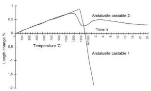
Fig. 12: Creep resistance of Andalusite based low cement castables at 1500 °C. Castable 2 with matrix aluminas (HCS at 1500 °C: 11 MPa), castable 1 without (HCS 1 MPa) [30]
