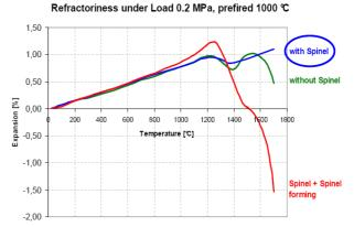
Fig. 10: Refractoriness under load (RuL) of tabular and spinel self flowing castables (samples pre-fired 1000  $^{\circ}C$  / 5 h)
