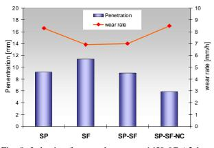
Fig. 8: Induction furnace slag test at 1650  $^{\circ}$ C / 2 h and CaO:Al<sub>2</sub>O<sub>3</sub> ratio = 1.08 (+ CaF<sub>2</sub>). Spinel (SP) and Spinel forming (SF) castables and combinations thereof; MgO contents between 4.5 and 6.3 %, open porosity at 1500  $^{\circ}$ C between 15.3 and 17.7 % [35]
