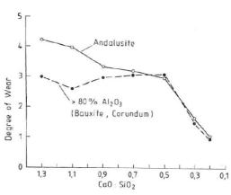
Fig. 3: Resistance of andalusite and bauxite / corundum bricks against slag with different CaO:SiO<sub>2</sub> ratio at 1520  $^{\circ}C$  / 4 h [27]
