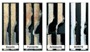
Fig. 6: Induction furnace slag test at  $1600 \text{ }^{\circ}\text{C} / 2$  h and CaO:Al<sub>2</sub>O<sub>3</sub> ratio = 1.08. Bricks of Andalusite, Bauxite, Forsterite vs. Bonite (dense CA<sub>6</sub>) castable [24]
