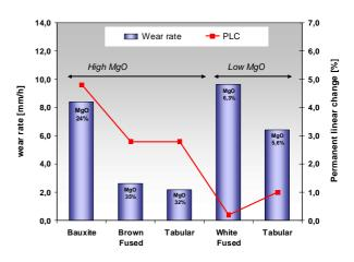
Fig. 9: Induction furnace slag test at 1650  $^\circ\text{C}$  / 2 h and CaO:Al\_2O\_3 ratio = 1.08 (+ CaF\_2). Resin bonded AluMagCarbon bricks with high and low MgO content. Permanent linear change is considerable higher with high MgO content
