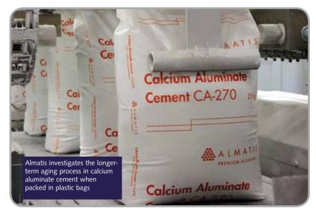
Cement in bags without a moisture barrier and any pallet protection also show an increase in water demand. Water demand remains stable for cement packed in bags incorporating a moisture barrier. For pallets covered with a stretch hood, the type of bag is of minor importance and cement parameters such as initial setting and water demand remain stable over the entire storage period.
