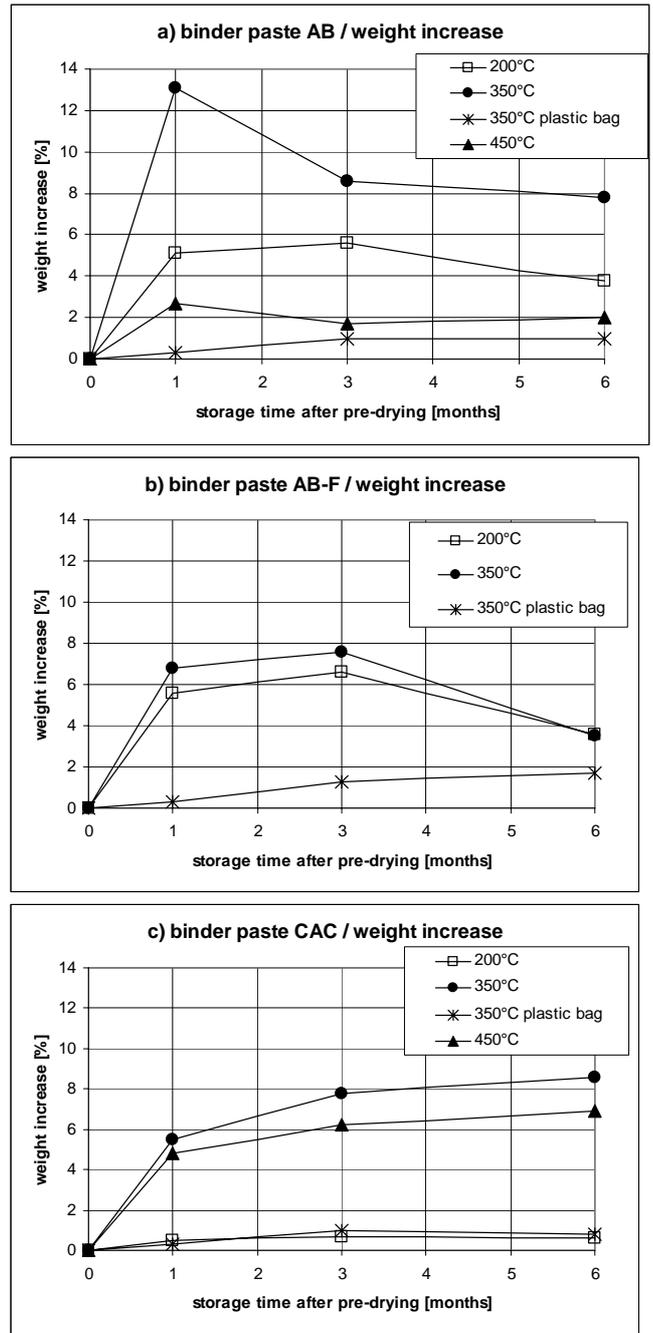
Fig. 4a-c. Binder paste test bars: Development of weight increase during storage period
