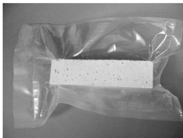
Fig. 1. Test bar packed in plastic bag for moisture protection
