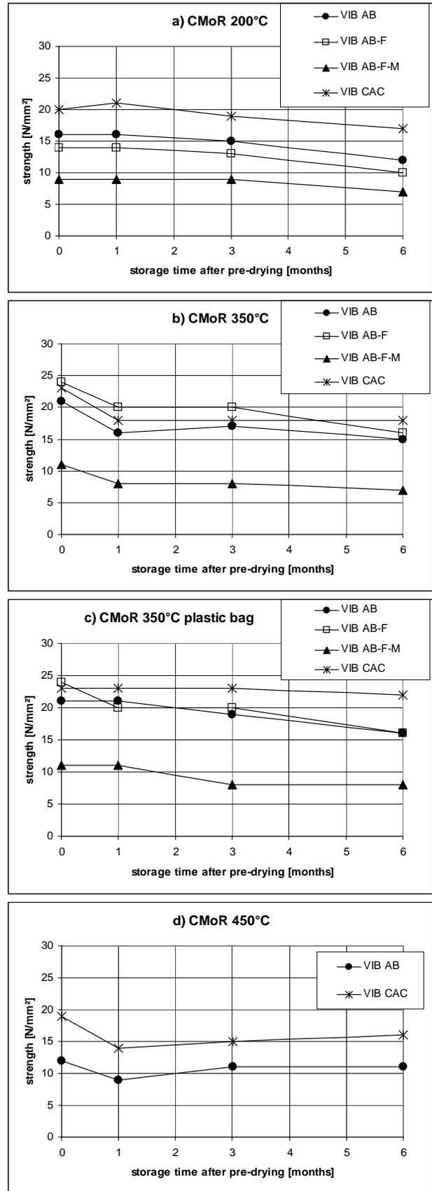
Fig. 2 a-d. Castable test bars: Development of Cold Modulus of Rupture during storage period
