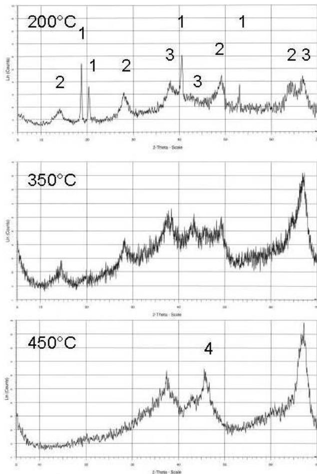
Fig. 5a-c. X-ray diffraction (5-70 degree 2-theta) from Alphasond binder paste pre-fired at 200, 350, and 450°C (5 hours each).
