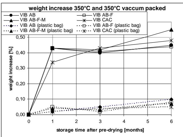
Fig. 3. Weight increase of castable test bars after drying at 350°C, with and without plastic bag protection. Weight increase as a result of moisture absorption during storage is reduced by plastic bag packaging
