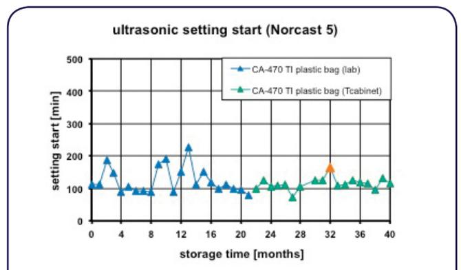
Figure 6: impact of warehouse aging of plastic bagged CA-470 TI on ultrasonic setting start. Measurement phase 1 (0 – 21 months) in the lab and phase 2 (22 – 40 months) in a temperature cabinet at 20°C (month 32 data point, see text)
