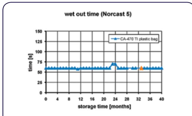
Figure 4: impact of warehouse aging of plastic bagged CA-470 TI on wet-out time (month 32 data point, see text)
