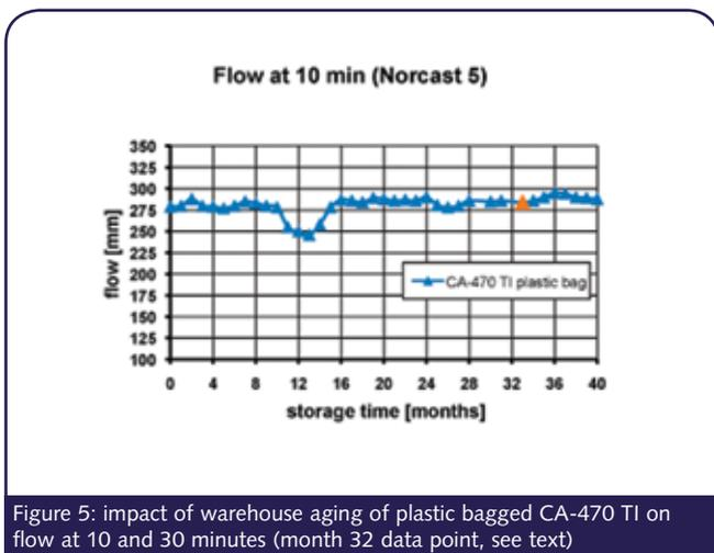
Figure 5: impact of warehouse aging of plastic bagged CA-470 TI on flow at 10 and 30 minutes (month 32 data point, see text)
