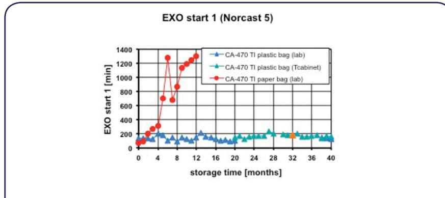
Figure 7: impact of warehouse aging of CA-470 TI on setting (EXO start 1), plastic versus paper bag. Measurement for CA-470 TI in plastic bags: phase 1 (0-21 months) in the lab and phase 2 (22-40 months) in a temperature cabinet at 20°C (month 32 data point)
