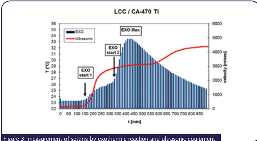
Figure 3: measurement of setting by exothermic reaction and ultrasonic equipment
