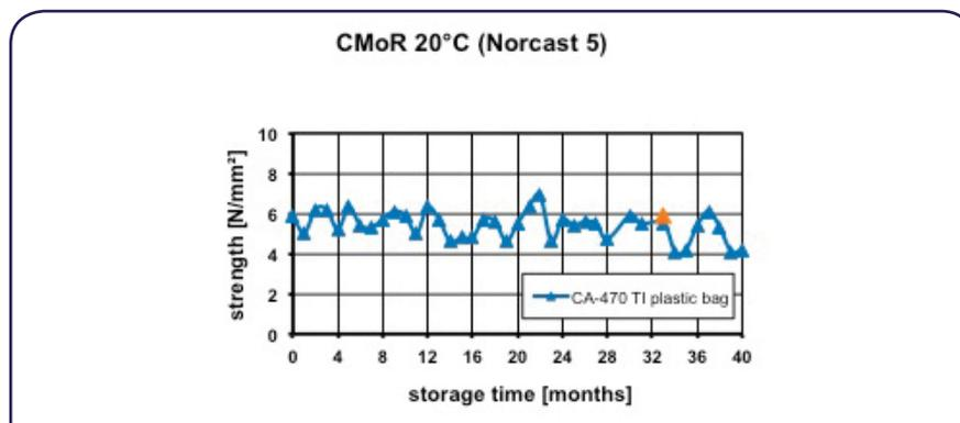
Figure 8: impact of warehouse aging of plastic bagged CA-470 TI on strength of test castable (CMoR 20°C) (Month 32 data point, see text)
