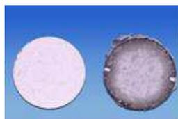
Fig. 7c: Test pieces of pure Bonite castable (BON 1) before (left) and after (right) aluminium resistance test. Test piece fired at 1400 °C before test.
