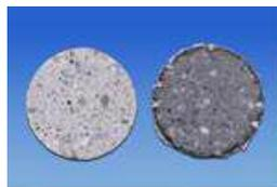
Fig. 7b: Test pieces of conventional bauxite castable (BX 1) before (left) and after (right) aluminium resistance test. Test piece fired at 900 °C
