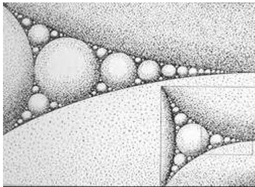
Fig. 1: Dense particle packing [13]. Voids successively filled by smaller particles to reduce water demand and enhance strength.
