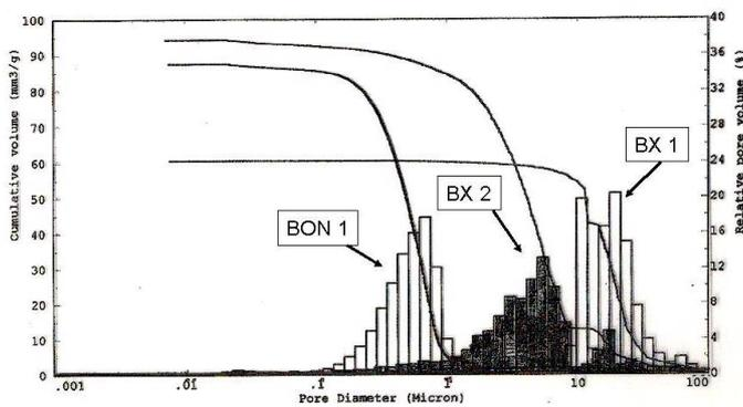
Fig. 3: Micropore size distribution (Hg intrusion method) of Bonite castable BON 1, bauxite/silica fume castable with  $BaSO_4$  (BX 1) and bauxite/alumina castable with  $BaSO_4$  (BX 2), all pre-fired for 5h at 1400 °C
