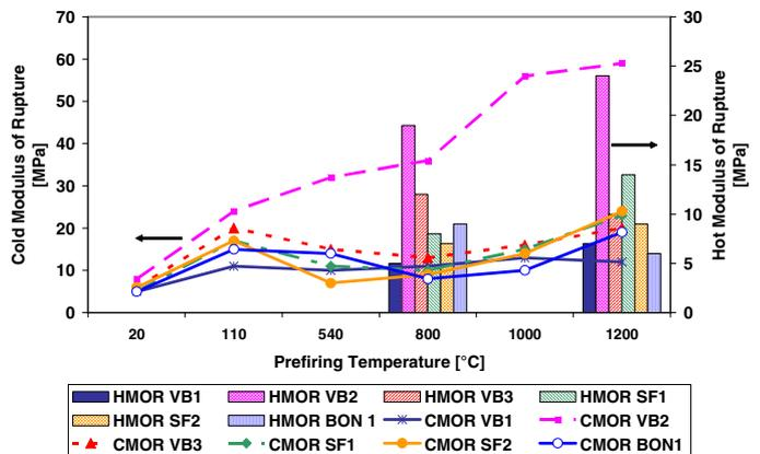
Fig. 5: Cold (lines) and hot (bars) modulus of rupture of test castables
