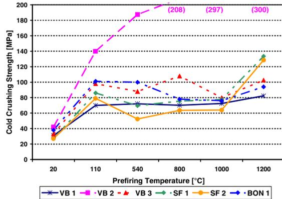
Fig. 4: Cold crushing strength of test castables after pre-firing at different temperatures
