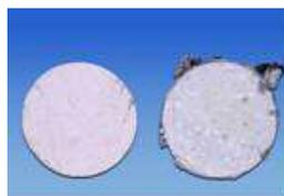
Fig. 7a: Test pieces of pure Bonite castables (BON 1) before (left) and after (right) aluminium resistance test. Test piece fired at 900 °C before test
