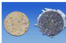
Fig. 7d: Test pieces of commercially available bauxite castable (BX 1) before (left) and after (right) aluminium resistance test. Test piece fired at 1400 °C before test.
