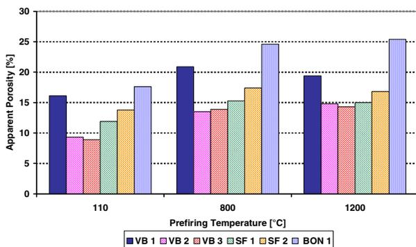
Fig. 2: Apparent porosity of test castables
