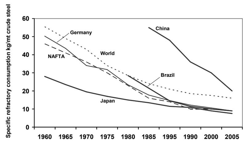
Fig. 5: Steel industry specific refractory consumption trend [8-12]
