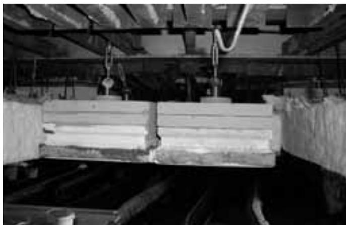
Fig. 4. Microporous pre-cast shapes for kiln roof, 400 × 350 × 160 mm with high alumina anchor brick and two 50 mm calcium-silicate plates on top [7]
