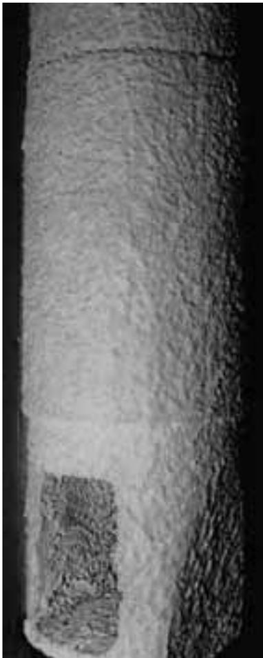
Fig. 3. Submerged nozzle with sprayed on microporous insulation on the surface and in the port holes [6]
