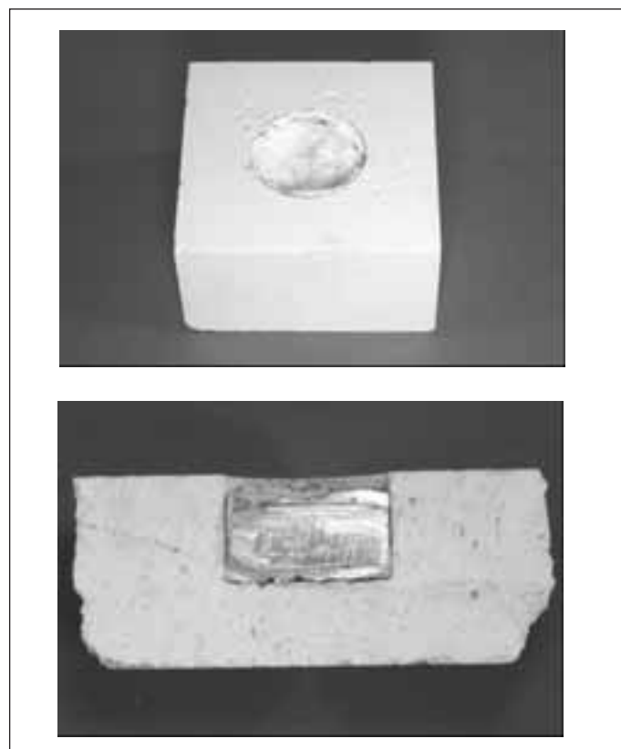
Fig. 1. Bonite test crucible after aluminium plus alkali salt resistance test (aluminium alloy AZ8GU, 45% KCl, 45% NaCl, 10% NaF)
