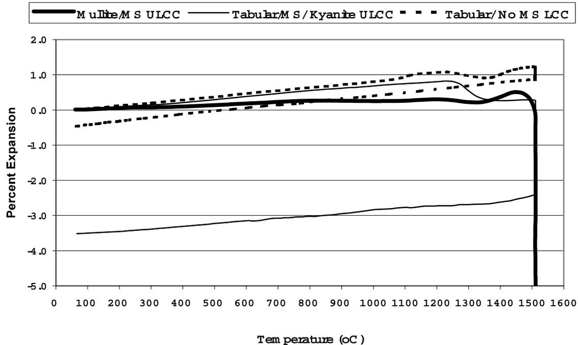
ASTM C-832 was used to determine Expansion Under Load (EUL) and Creep Under Load (Creep) for each test castable. These tests were run at the Orton Foundation Laboratory on dried samples. The results for EUL are plotted in Figure 6 and in Figure 7 for Creep.
