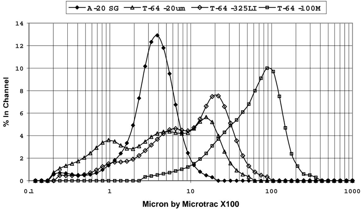
Figure 2: Typical Multi-modal Matrix Aluminas
