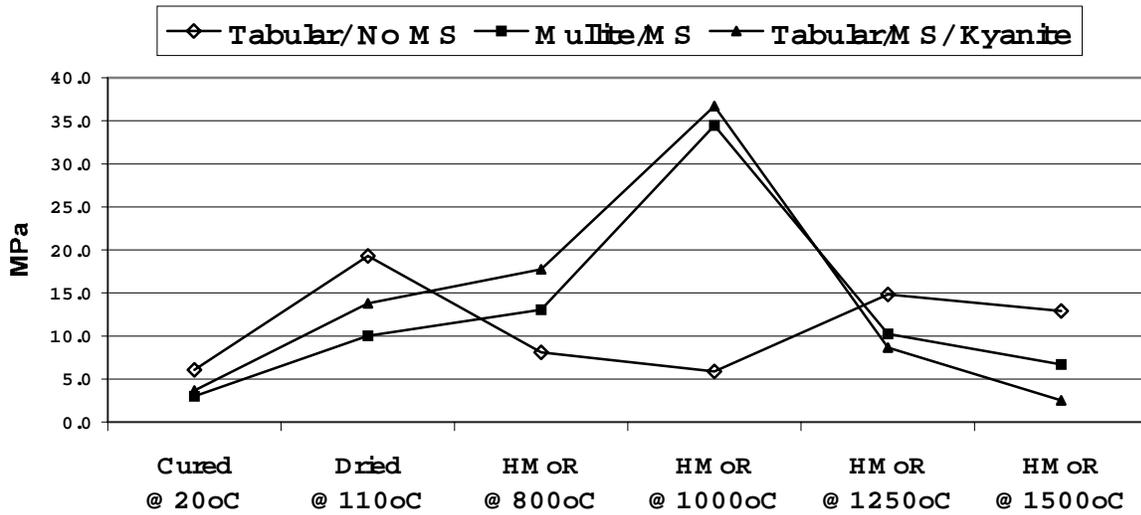
ASTM C-133 was used to determine Modulus of Rupture (MoR) after (1) curing 24 hours at ambient (20°C) temperature in a sealed plastic bag and (2) drying 24 hours at 110°C. Hot Modulus of Rupture (HMoR) was evaluated using ASTM C-583 at 800, 1000, 1250, and 1500°C. The results are plotted in Figure 5.
