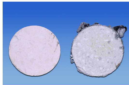
Fig. 5 a: Test pieces of pure Bonite castable (BON 1) before (left) and after (right) aluminium resistance test. Test piece fired at 800°C before test
