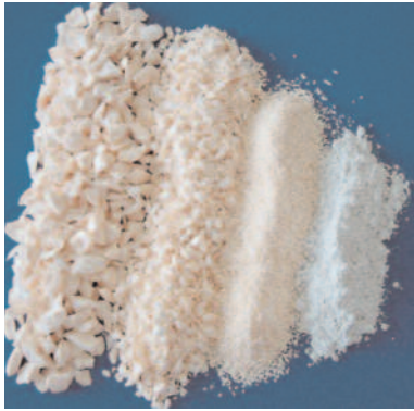
Fig. 2 a, b Dense calcium hexa-aluminate BONITE product line
