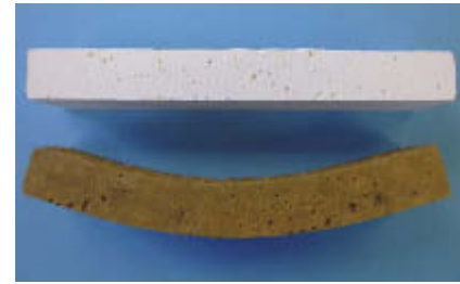
Sag test of castables at 1,550° C/ 5 hours. Tabular/Spinel castable shows no deformation versus bauxite castable which forms liquid phases and shows deformation.
