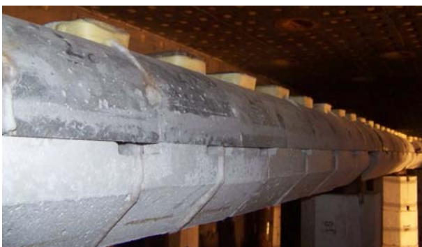
Fig. 7: Top shells made of dense castable on the upper side of the skids, light weight shells on the bottom side
