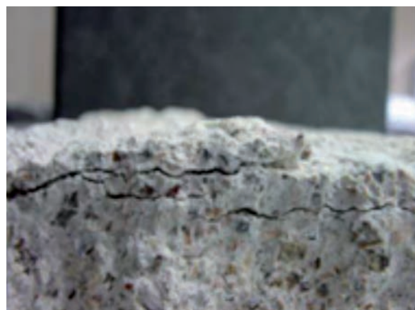
Fig. 2 Spalling of incinerator lining due to alkali corrosion [16]
