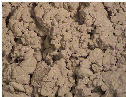
Fig. 2: Castable wet out time end point in a laboratory mixer
