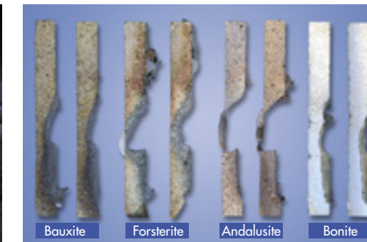
Bonite corrosion resistance against steel slag
